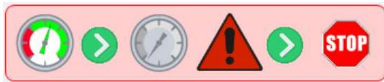
With this selection, if the pressure drops below the minimum threshold, the machine stops, the valve is closed and the pressure alarm is triggered. The machine goes into a STOP status and can only restart after an operator has intervened.
