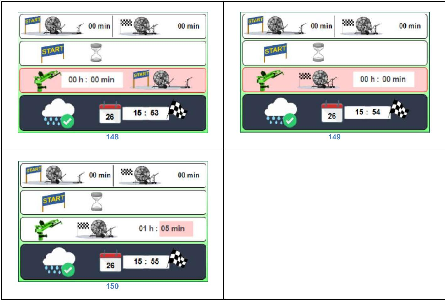
Through the first setting it is possible to define whether the second raingun must operate for the set time (figure 70) in the starting stage (trolley fully out figure 68) or in the stage near the end of operations (trolley near the machine figure 69)
