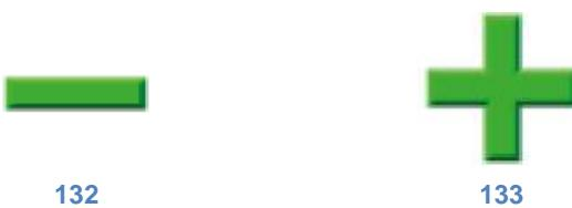
If none of the two symbols are visible, this means that the ByPass valve is not controlled at that time.
