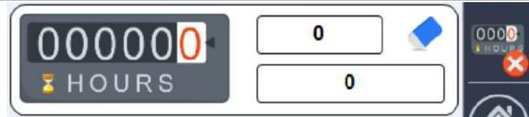
the first value (next to the rubber) represents the partial hour counter which can be reset by pressing and holding the F7 key for at least 5 seconds, the first password level is also required. The second value represents the overall hours worked by the machine which are reset only if the serial number is modified.
