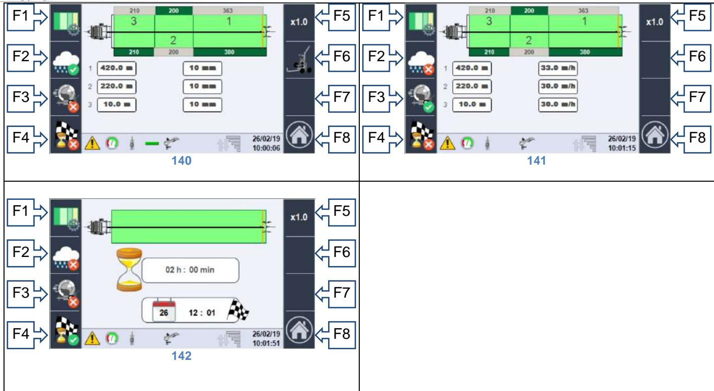
Based on the active operating mode, one of the above pages can be accessed. The machine's work field is represented schematically in the top part of all pages, the maximum irrigable length is given by the length of the hose, while the actual trolley position is given by the yellow line near it. At the edges of the field it is possible to see the length of every single sector relating to the overall length of the field (in green) or to the position of the trolley (in grey).
