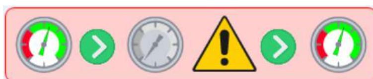
With this selection, if the pressure drops below the minimum threshold, the machine stops, closes the inlet valve and waits for the pressure to increase again, above the minimum threshold, to reopen the valve and start the cycle again (the machine remains in the START status). There are no limits to the number of stops.
